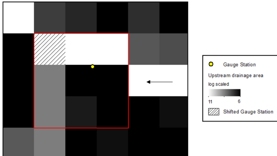
Figure 3-2 Shifting algorithm employed in the 30" data set for outlet locations representing gauge stations and reservoir locations.
